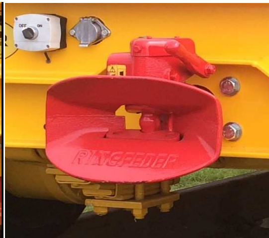
Coupling Closed (Pin Locked)
