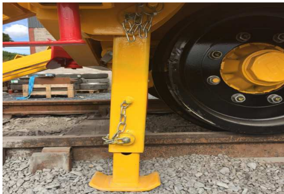
Jack legs in loading/Unloading position
