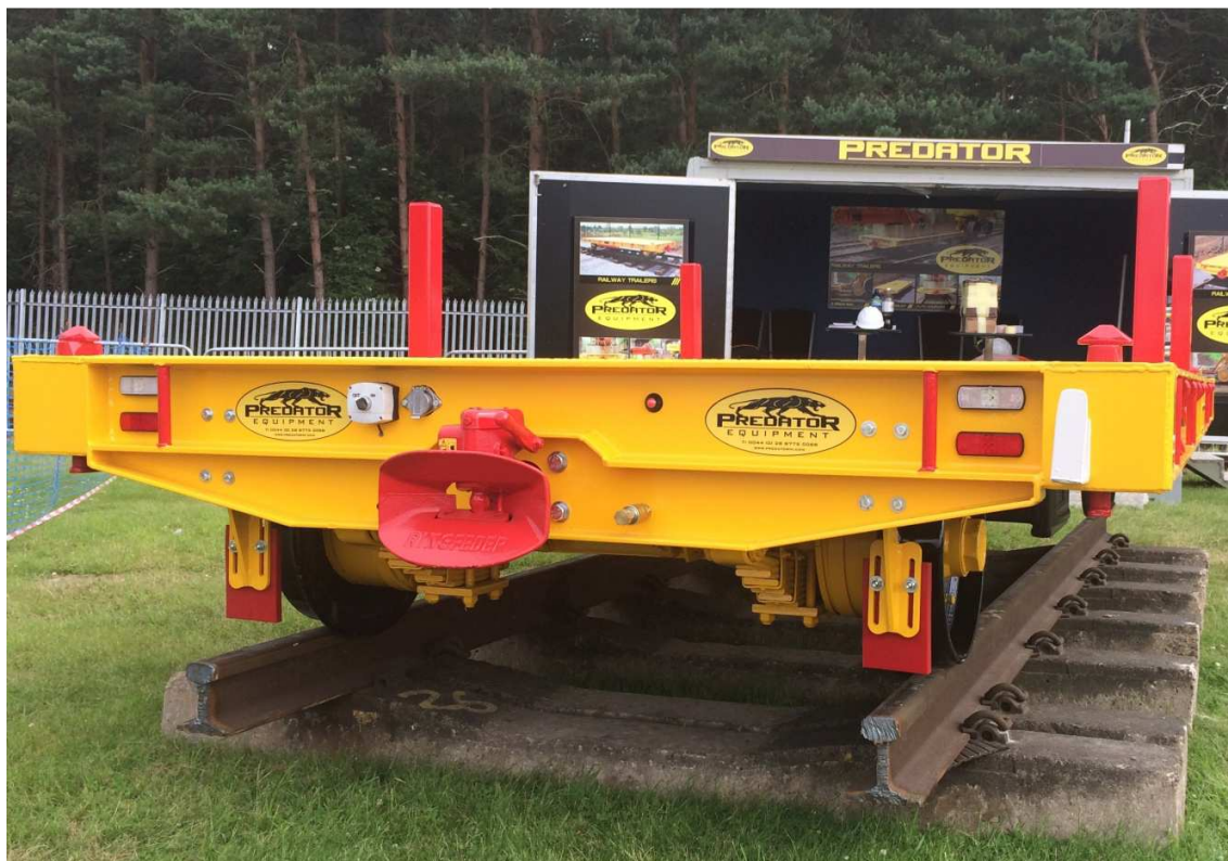
Rail Scrapers attached to the trailer headboard.
