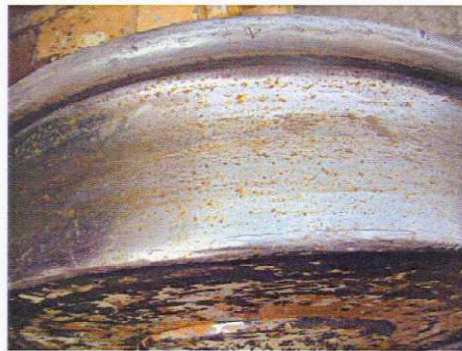
Figure 7 - Circumferential cracking associated with rollover
