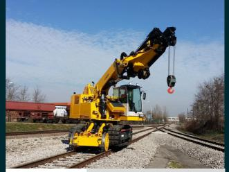
Weight Length Width Mast Reach 42 tonnes 10.5m (Rail Configuration - Extended) 9.2m (Road Transport Configuration) 2.7m (height) 3.5m 15.2m
